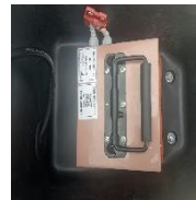
3. Disconnect Battery Power Plug Socket
