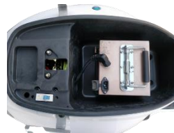
3. Disconnect Battery Power Plug Socket
