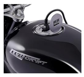
The charger provided with the Li-Ion battery is sophisticated and is a special purpose electronic charger. This charger has an additional safety feature which provides protection from output overvoltage, output overcurrent and short-circuit. The charger is designed to charge only ecoDryft<sup>®</sup>.
